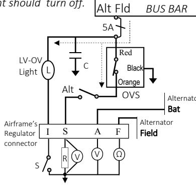
With the master switch on, the voltage on the alternator BAT post and the voltage on pin A should be the same. Turn off the master switch.
