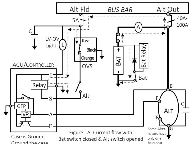
If the pin S voltage is less than bus' but not 0 Volt:
