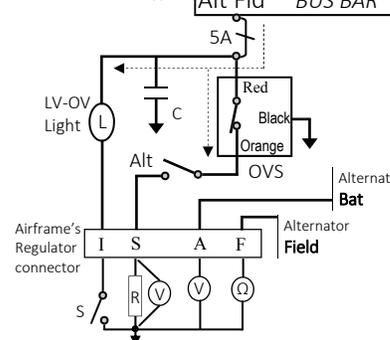
With the master switch on, the voltage on the alternator BAT post and the voltage on pin A should be the same. Turn off the master switch.
