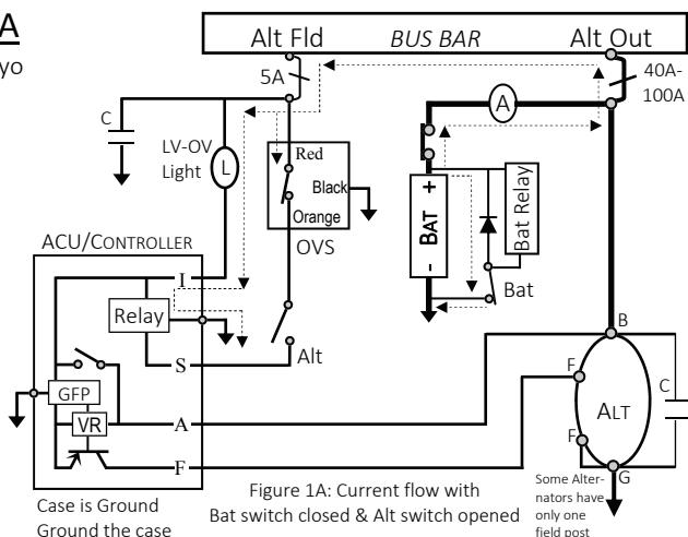
Except for step 5, take all measurements with the engine off. Take the step 5 voltage from the bus (inside) away from the propellers. It is easier to take the measurements in steps 1 to 4 with the unit unbolted from the firewall, its case grounded to the firewall. This will allow easier access to pins I, A, S, and F, as well as, prevent grounding any of the pins.
